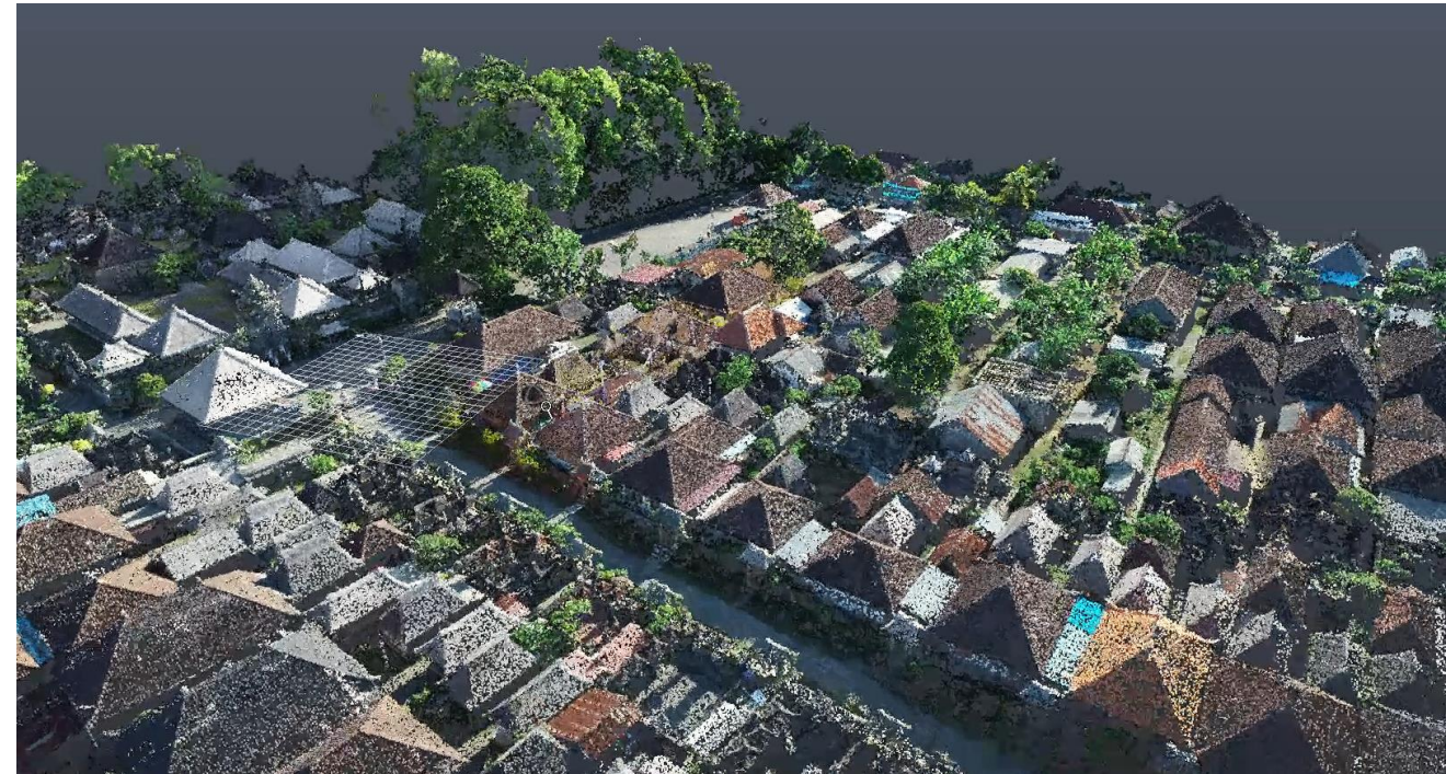
Integration of point clouds from TLS and Orthophoto RMSE = 0.003m or 3 mm
