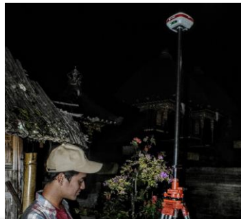
Gnss Observations (3 hours) – (E=0,3mm, N=0,3mm, H=1mm)
